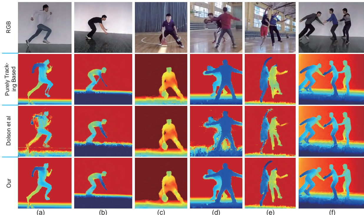
Fig. 9. Reconstructed depth map of real-world scenarios. From top to down rows: input color images, depth maps reconstructed by the purely tracking based method, results by Dolson et al’s method [12], and results by our method.
